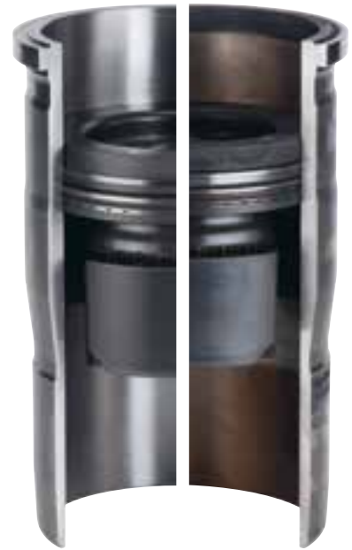
Before (left) and after 1.2 million kilometers (right): the MAHLE components had survived the prolonged stress unaffected.
