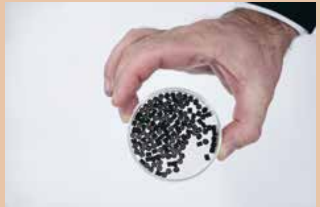
Elegant and efficient: these activated carbon parts bind gasoline vapors.
